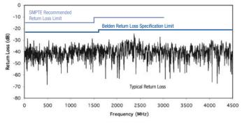
Belden's extremely popular HDTV Brilliance® Broadcast video cables are now 4.5 GHz sweep tested! Prepared for 1080p formats, 1855, 1505A, 1694A and 7731A cables are sweep tested to 4.5 GHz. Belden has always tested every finished put-up to be certain of a top quality product. This is the only way in which damage introduced in finishing operations can be detected. This process sets Belden apart from competitors who only test in batches.
