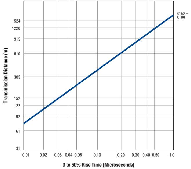
Cables are terminated in their characteristic impedance. Signal source electrical characteristics: 50 Ohm and 10% to 90% rise time less than 5 nanoseconds.
